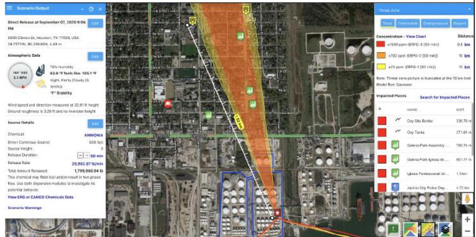
Access live meteorological data for modeling by selecting nearby internet weather stations or user provided local fixed or portable met stations and compare model results against gas sensor concentrations.
